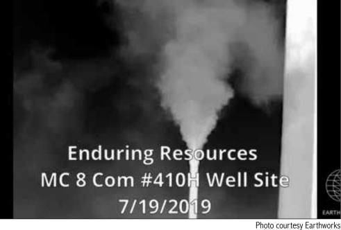
Research tying public-health impacts to oil and gas development in New Mexico is increasing. Earthworks thermographers are using infrared cameras to find leaks of methane and volatile organic compounds at oil and gas wells. This camera shot shows a leak of methane and volatile organic compounds, invisible to the naked eye, near **Counselor on the Navajo Nation.**
