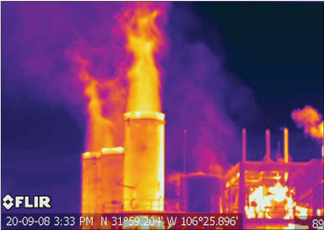
Earthworks used its optical imaging cameras at Newman Gas Plant in northeast El Paso, above, to make visible the normally invisible pollution of volatile organic compounds escaping and traveling to surrounding communities.
